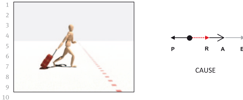
11 Fig. 2: A free-body diagram (on the right) showing how the dynamics model would specify the 12 force dynamic situation depicted (on the left). A = the affector force, P = the patient force, 13 R = the resultant force, E = endstate vector, which is a position vector, not a force.
